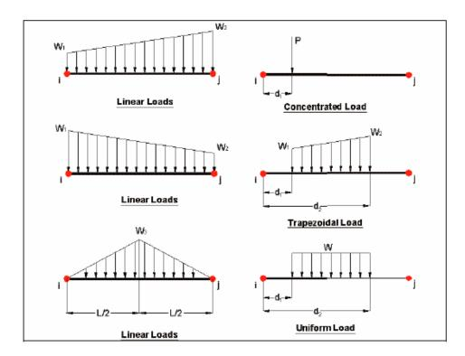
Fig 3.3: Member load configuration
