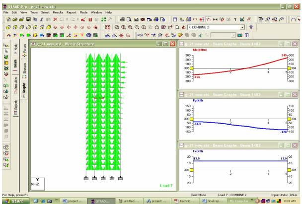
Fig 8.4: graph for shear force and bending moment for a beam
