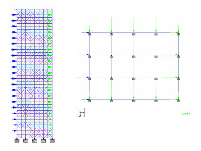
Fig 4.11: wind load effect on structure elevation and plan
