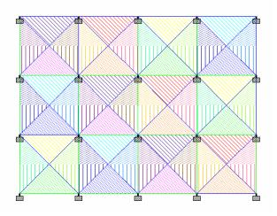
Fig 4.7: load distribution by trapezoidal method
