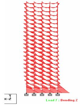
Fig 8.2: bending in  $\boldsymbol{Z}$
