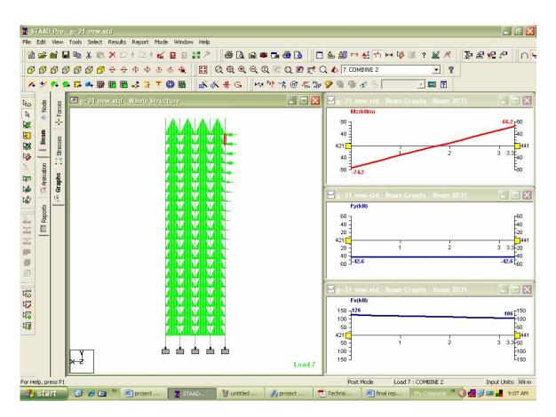
Fig 8.5: graph for shear force and bending moment for a column
