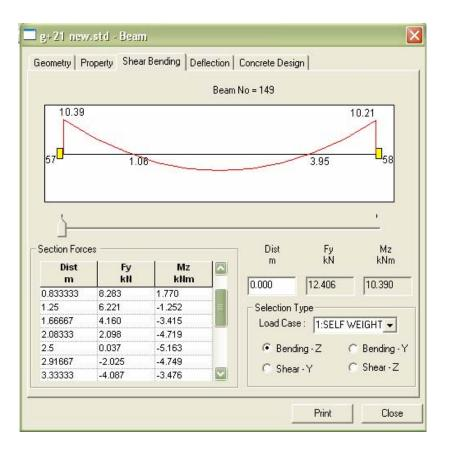
Fig 7.3: Shear bending of beam no. 149
