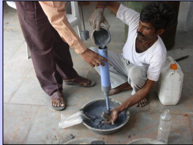
Pump made from plastic pipes and nozzle
