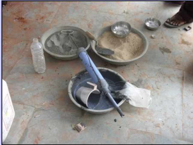
Pump made from plastic pipes and nozzle
